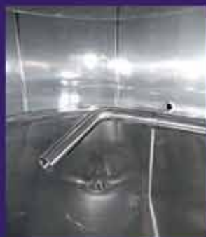
Inside view of stainless steel racking decanting arm
